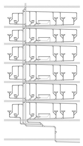
Figure 68: Drainage system with branch ventilation of the sanitary appliances
