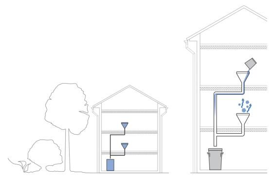
Figure 2: Building drainage around 1850
