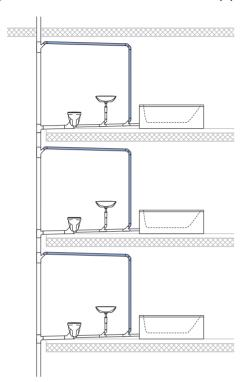
Figure 37: Branch ventilation pipe
