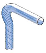
Figure 46: Flow conditions in the Geberit HDPE BackFlip bend
