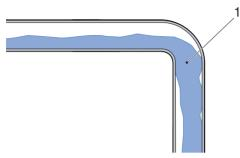
Figure 42: Hydraulic blockage when the direction is changed from horizontal to vertical
