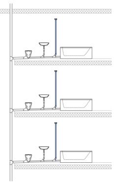
Figure 38: Pipe with air admittance valve
