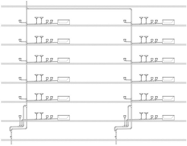
Figure 64: Drainage system with collective ventilation
