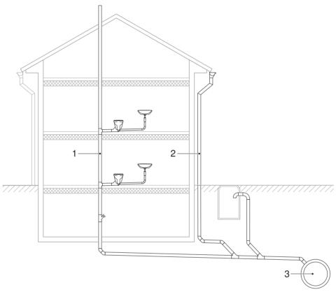
Figure 12: Structure of a combined system
