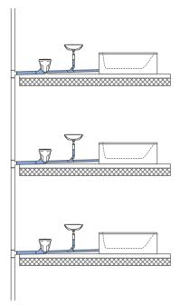
Figure 30: Branch discharge pipe per floor
