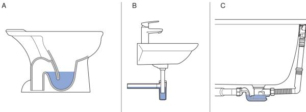
Figure 27: Trap designs for sanitary appliances
