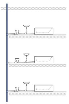
Figure 35: Main ventilation pipe
