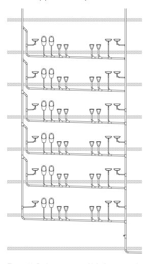
Figure 66: Drainage system with indirect secondary ventilation
