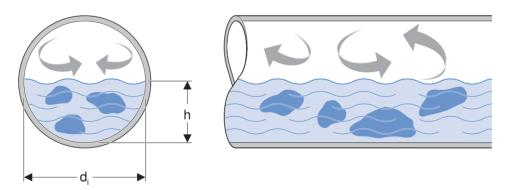
Figure 16: Optimal filling level in horizontal pipe sections
