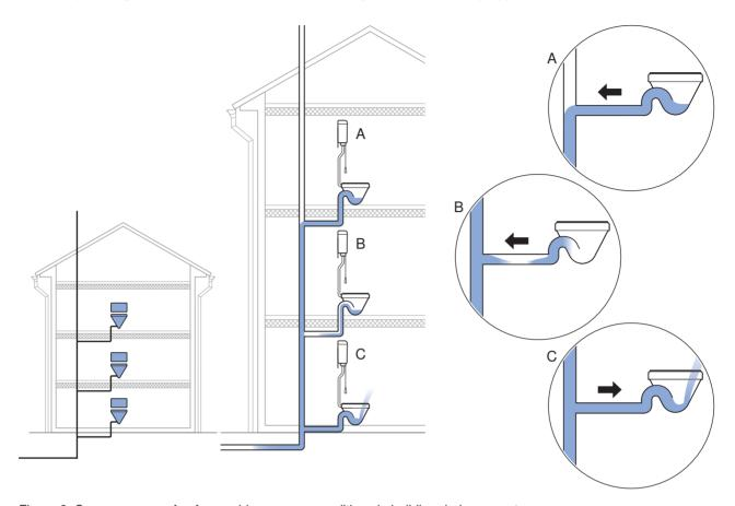
Figure 6: Consequences of unfavourable pressure conditions in building drainage systems
