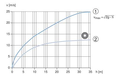
Figure 25: Theoretical falling velocity and falling velocity in stacks
