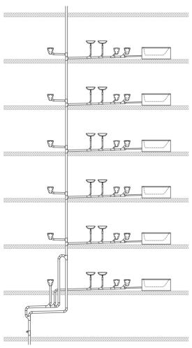
Figure 63: Drainage system with individual ventilation
