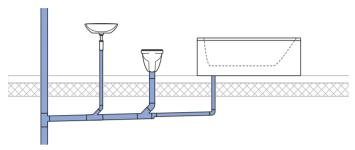
Figure 74: Laying the branch discharge pipe under the ceiling, single stack
