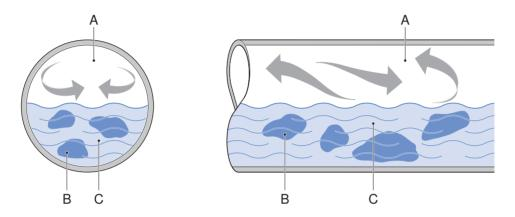
Figure 14: Transported substances in a partially filled discharge pipe
