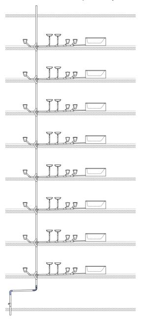
Figure 69: Drainage system with Geberit SuperTube
