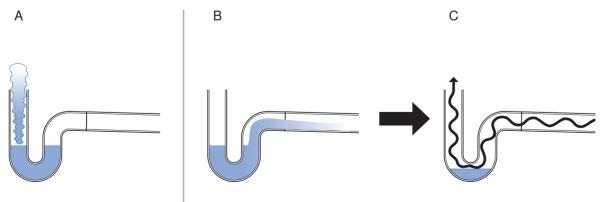
Figure 29: Causes which reduce the water seal depth
