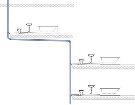
Figure 32: Stack with stack offset
