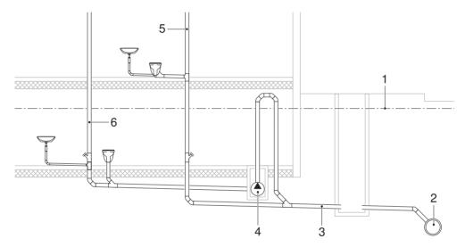
Figure 61: Preventing backpressure with a faeces lifting system
