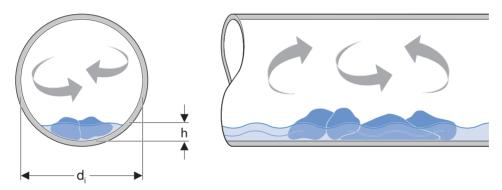
Figure 18: Too low a filling level in horizontal pipe sections
