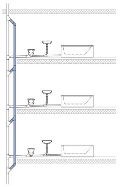
Figure 36: Secondary ventilation pipe
