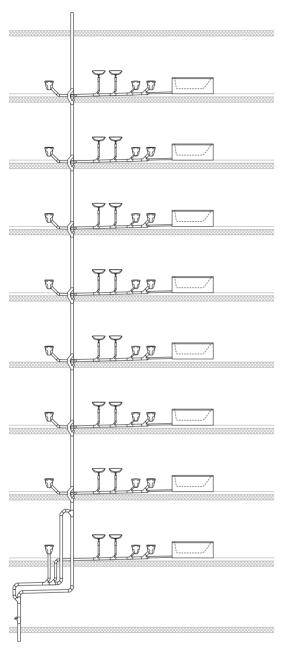
Figure 70: Drainage system with a Geberit HDPE Sovent fitting d160
