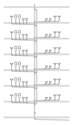
Figure 65: Drainage system with direct secondary ventilation
