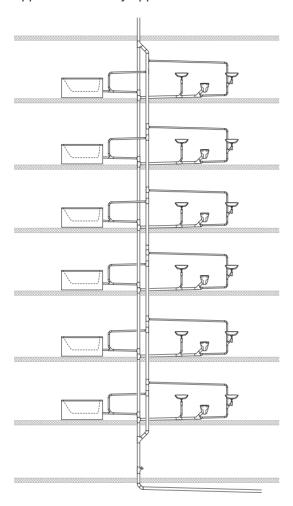
Figure 67: Drainage system with branch ventilation of the branch discharge pipes
