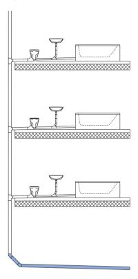
Figure 33: Underground and collector pipe
