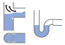
Figure 47: Flow conditions in an equal branch fitting 88.5° in the stack
