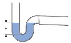
Figure 28: Water seal depth H according to DIN EN 12056-2:2001-01
