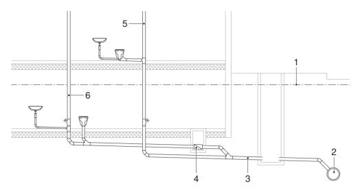
Figure 62: Preventing backpressure with a backpressure seal
