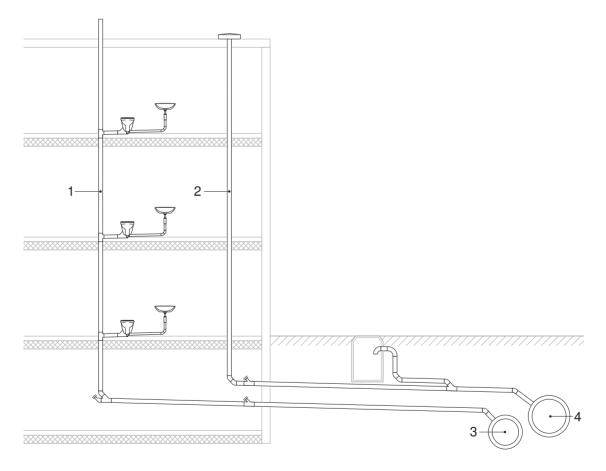
Figure 11: Structure of a separate system
