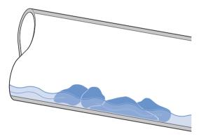
Figure 20: Too high a slope for the horizontal pipe section
