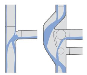
Figure 51: How the Geberit HDPE Sovent fittings function in comparison to conventional main vent stacks
