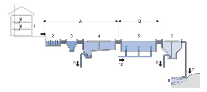
Figure 13: Sample structure of a waste water treatment plant
