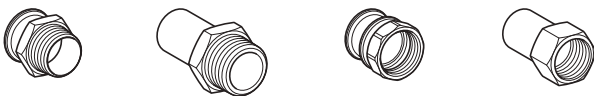
Figure 49: Geberit Mapress Carbon Steel adapters with male thread and adapters with female thread
