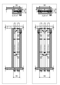
Planning with 3 parallel stacks consist of soil pipe, waste pipe and ventilation pipe
